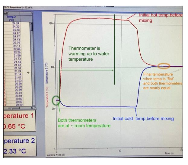
A typical experiment is above. When recording started both thermometers were at room temperature.
