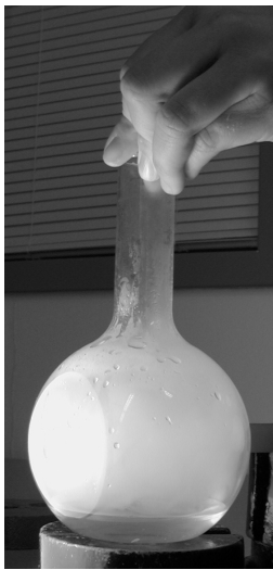
Figure C-13: With an understanding of how temperature and humidity interact, it is possible to make a cloud in a bottle.
